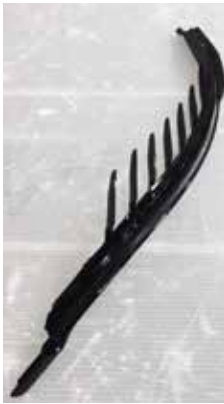
Super visible part, high glossy lightguide holder, produced on a Zhafir ZERES 3600/830 mady by PC in 40 s
